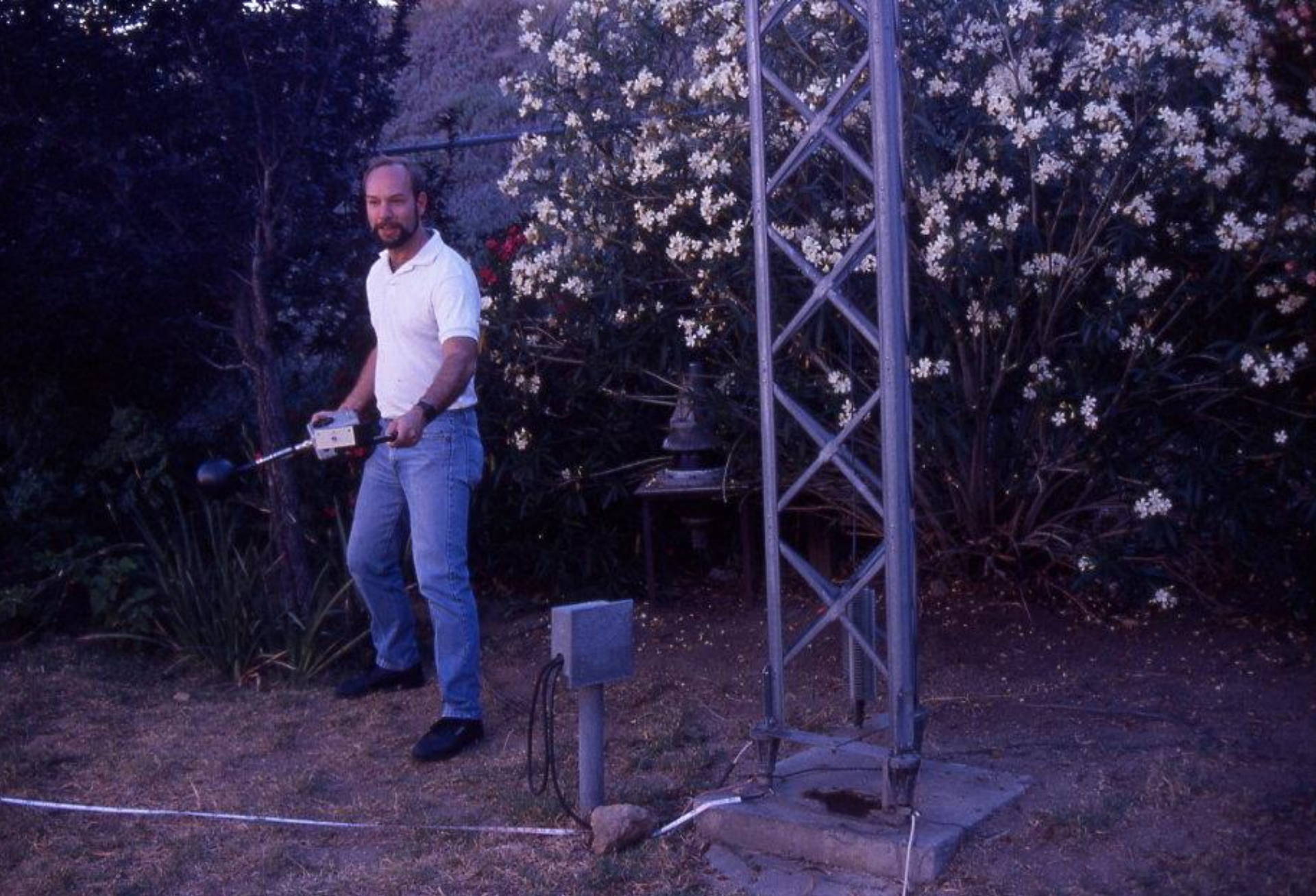
Measuring field near base of vertical antenna
