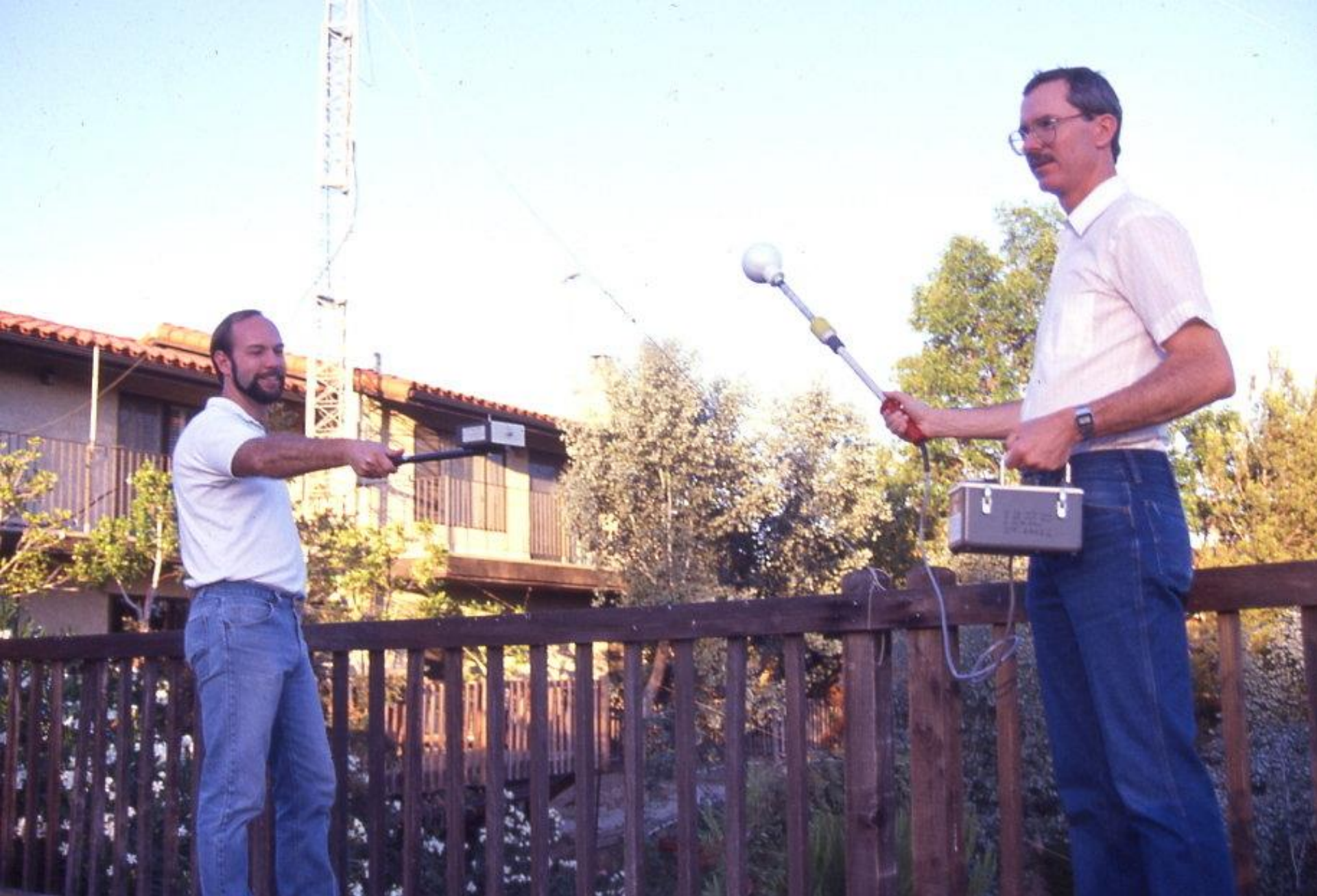
Measuring HF Yagi on tower at 75' (Ed Mantiply, EPA, and Bob Cleveland, FCC)
