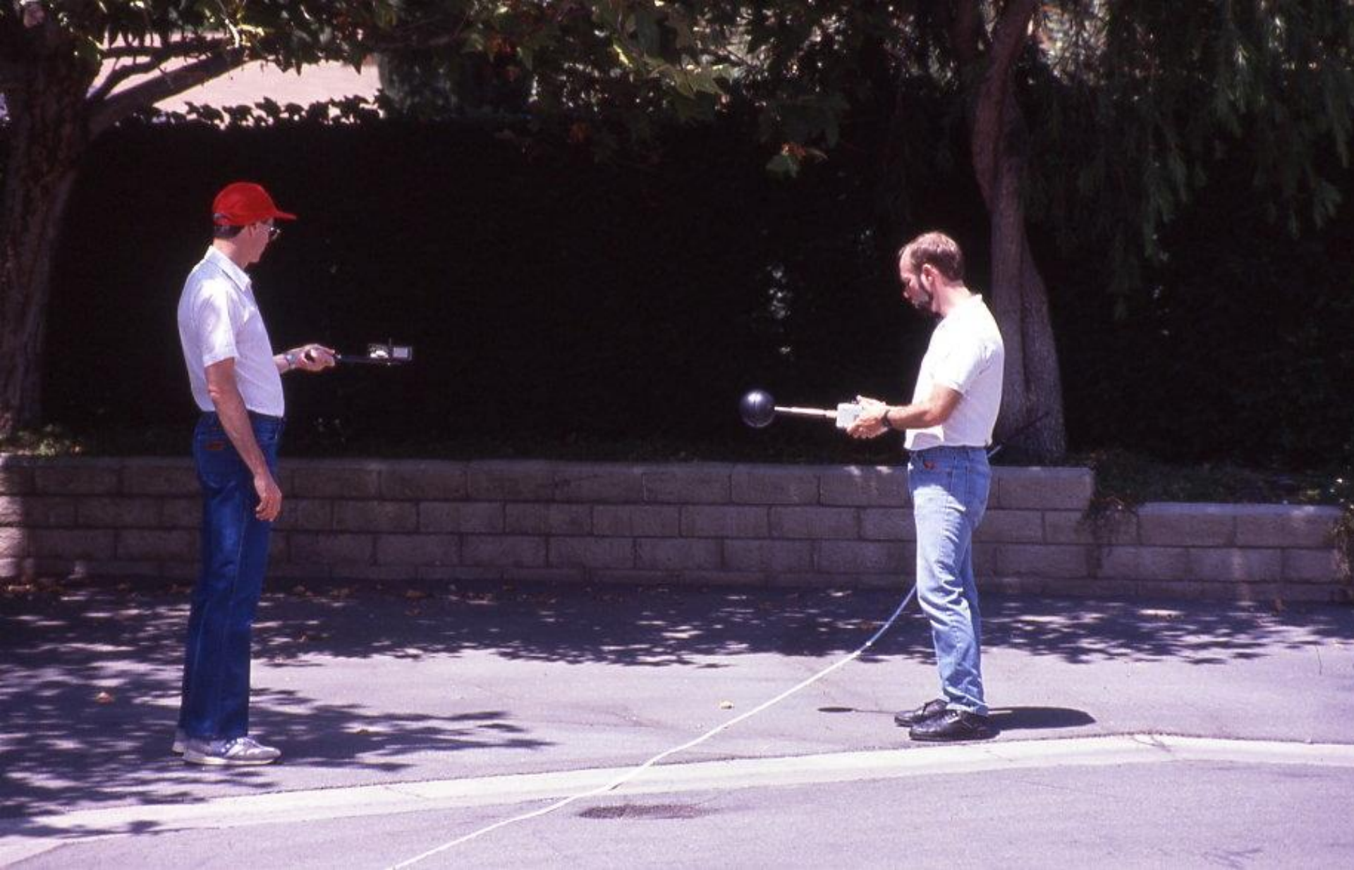
Measuring RF field near antenna hidden in tree
